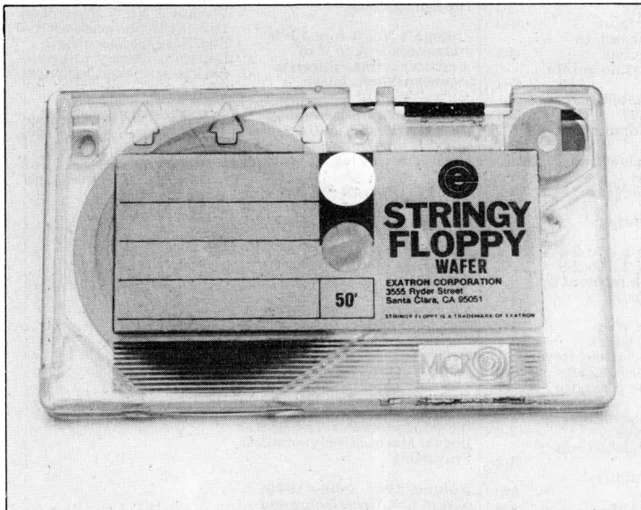
Facing page: The stringy floppy drive. Above: A wafer. Below: Inside the wafer, showing the tape being drawn from the centre of the spool and rewound on the outside.
